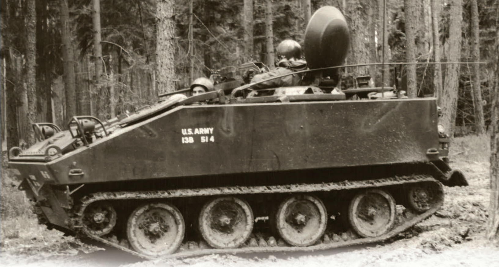
The M114. Initially considered an ideal scout platform due to its combination of armored protection and relatively small size, in fact the vehicle suffered from mobility constraints and poor operational readiness rates. (U.S. Army photo)
