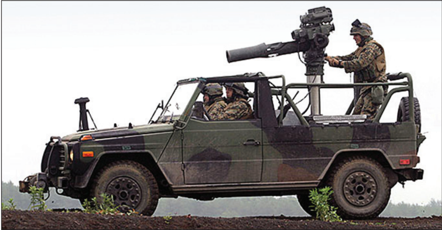
Figure 5. U.S. Marines in the intermediate fast-attack vehicle with a tube-launched, optically-tracked, wire-guided missile system. (Photo by U.S. Marine Corps)
