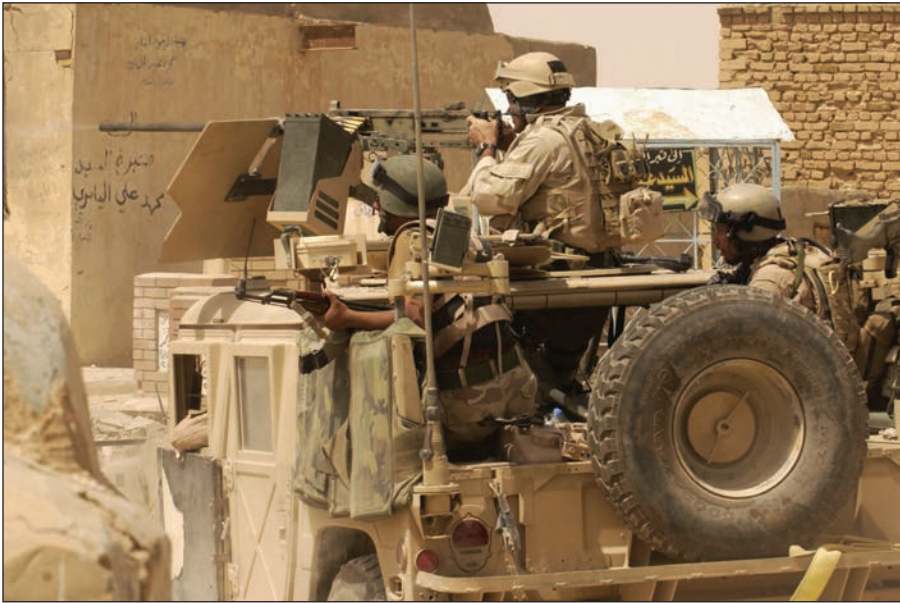
An armored humvee of 1 st Cavalry Division during the fighting in An Najaf. The gunshield and added ballistic protection improved crew survivability at the cost of scout mobility. (U.S. Army photo)
