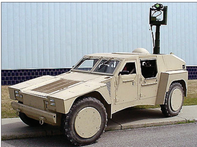
Figure 4. The Shadow RSTV with 4x4 hybrid electric drive. (General Dynamics Land Systems illustration)
