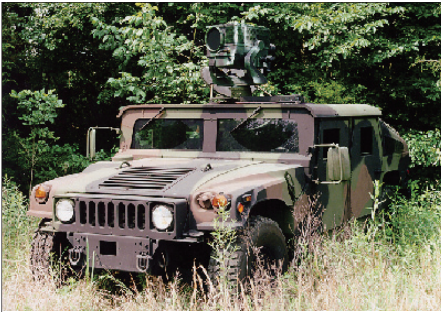
A humvee equipped with the Long-Range Advanced Scout Surveillance System. This device's ability to see targets at great distances encouraged the notion that scouts could develop situations from afar. (U.S. Army photo)
