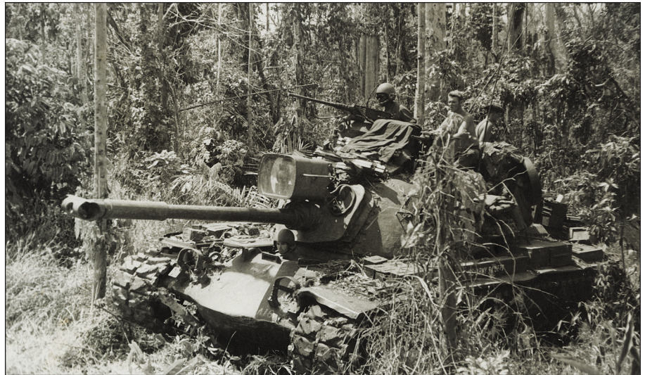
The M48A3 also had a 90mm M41 main gun which could fire 62 rounds of ammunition of varied types, including armor-piercing, high-explosive, anti-personnel canisters (pellets-flechette) and white phosphorus (for marking targets). (U.S. Army photo)
