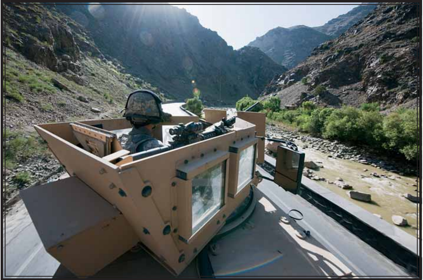
“The current standard issue, forcible entry, mounted platoon vehicle platform (M1151/M1167 variant HMMWV) in the reconnaissance squadron is incompatible with the long-range advance scout surveillance system (LRAS3) and improved target acquisition system (ITAS). The turret on both HMMWV variants and the mine resistant, ambush protected (MRAP) vehicle are not designed to accommodate the above-mentioned systems without modification, which requires considerable investment of unit operational and maintenance funds.”
