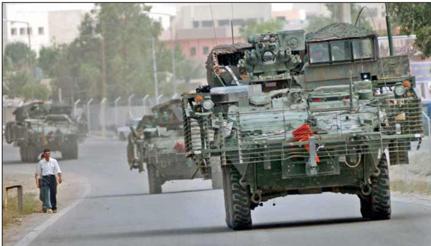
“In recent years, the U.S. Army developed and fielded the Stryker brigade combat team (SBCT). The SBCT is built around a digital network that shares situational awareness with all commanders at all levels simultaneously. The brigade is mounted in the Stryker family of vehicles, which are medium weight, extremely mobile, wheeled, and armor protected. They have proven to be ideally suited for combat in Iraq.”
