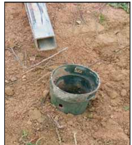
Figure 2. Green bag artillery powder canister dug into ground to serve as target base
