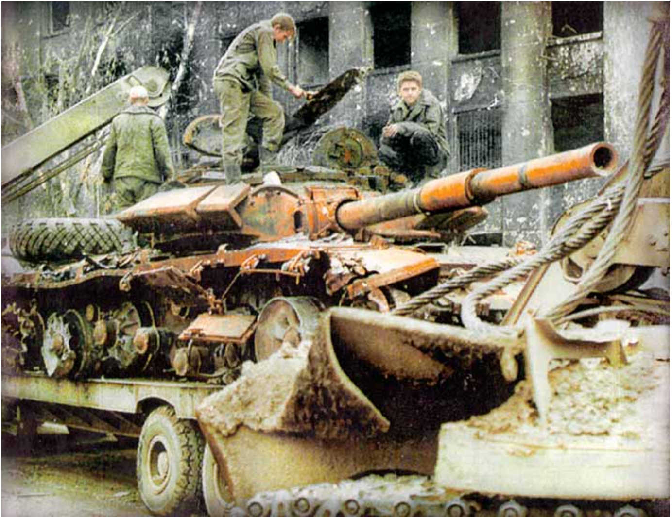
“Russian T80 tanks in the Battle for Grozny during 1994 and 1995 were equipped with reactive armor but proved vulnerable to the Chechen rebel tactics, which included volley fires of rocket-propelled grenade (RPG)-7 or RPG-18 rounds from overhead positions. Initial rounds would blow off the reactive armor panels, allowing subsequent rounds to penetrate. The Chechens also aimed for TC and driver hatches, knowing that these were particularly vulnerable points.”
