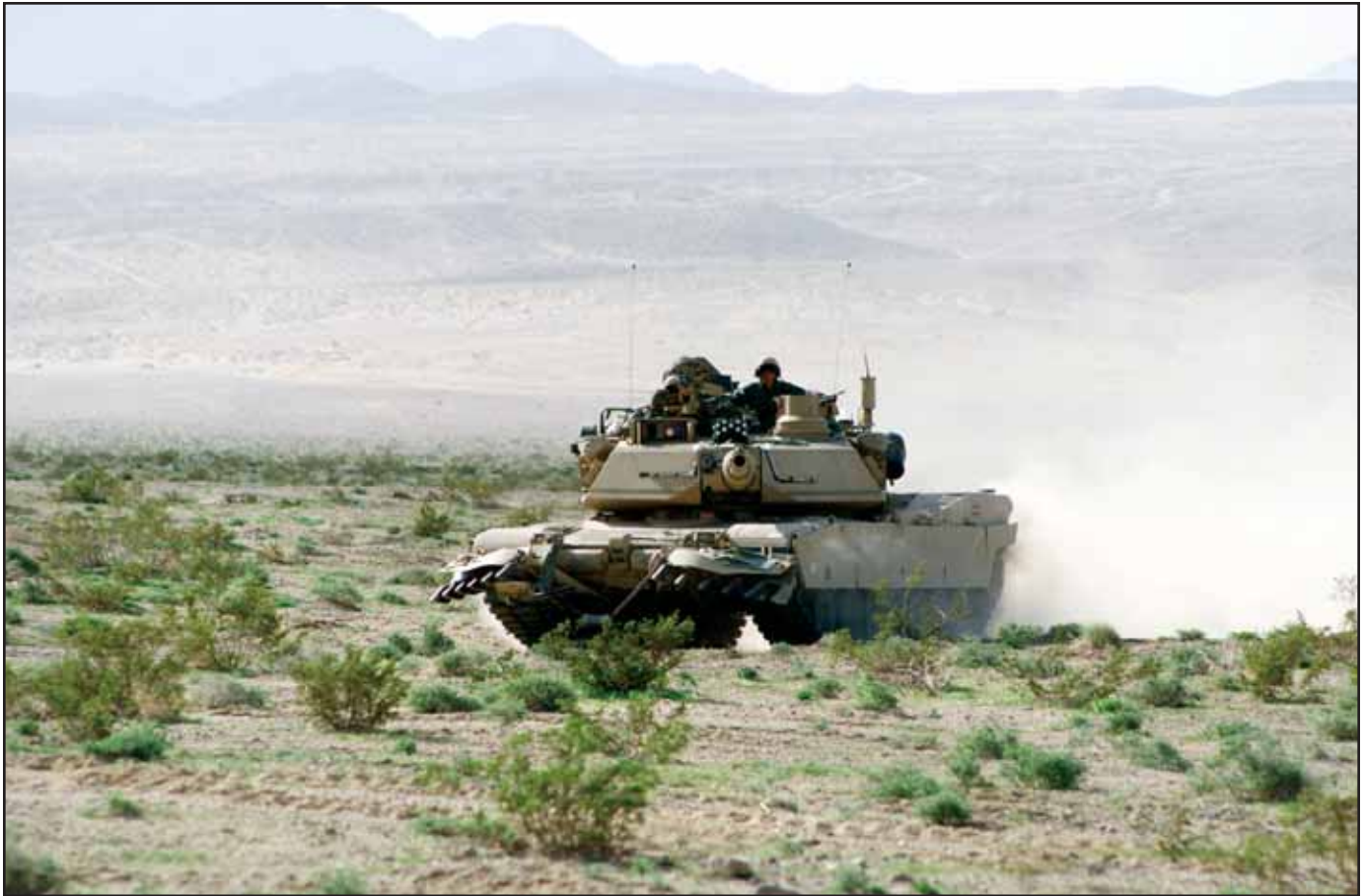
"The firepower of the M1-series tank is almost without peer today, but it was not intended for the urban battlefield. One key limitation is main-gun elevation and depression. M1 tanks are designed with low profiles; accordingly, the interior size of the turret is limited."
