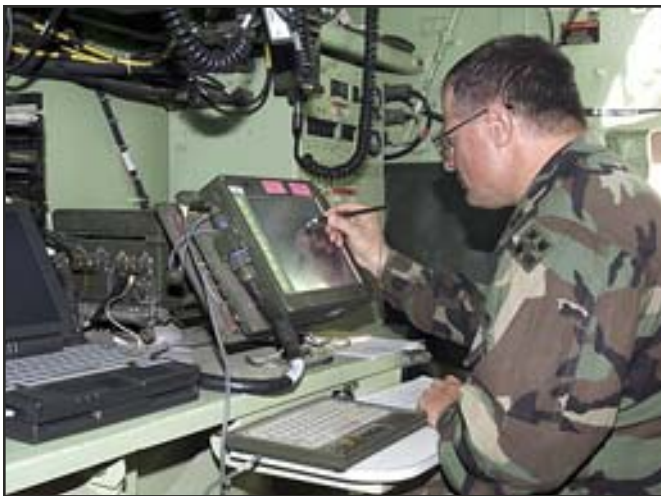
"FBCB2 mounted inside the Stryker helps the crew maintain situational awareness and their presence is populated on the squadron common operational picture within the TOC, thus enabling effective command and control. In the confined space of an urban area, with many dismounts operating in and around vehicles, fratricide prevention is a key concern."
