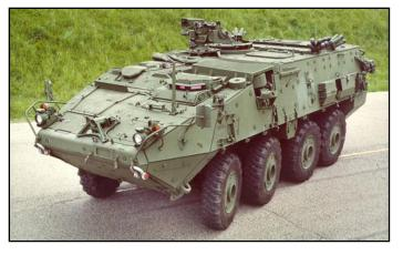
The standard appliqué armor on the LAV III does not protect against hand-held antiarmor weapons like the RPG-7 — the primary threat in urban combat. The author argues for additional protection from kits that would withstand attack from RPG-type HEAT warheads (Photo: GM Defense)
