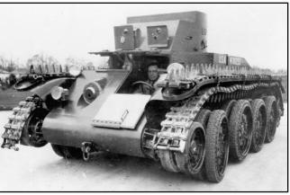
Above, the unusual Christie convertible wheel/track suspension is seen in the wheeled configuration with its tracks stowed above and below the fenders on each side. Called "combat cars" (the cavalry was prohibited from owning "tanks"), the T4 was armed with machine guns.
