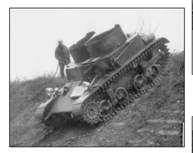
Above, the Ordnancesponsored T5 Combat Car descends a slope during testing. Its vertical volute spring suspension was later a common feature of U.S. light and medium tanks, but the idea of twin turrets was abandoned for tactical reasons.
