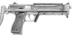
hits with a pistol, but their design and construction is such that they tend to be difficult and time-consuming to affix to the weapon, especially when the shooter is under stress. A proper PDW should be built with an integral folding or telescoping stock that is configured for rapid and easy deployment.
