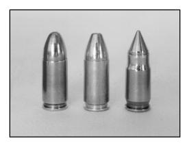
Penetration capability of current service pistols could be greatly increased by switching from standard 9mm ball ammo (left) to a hard-core, very high-velocity 9mm round (center), or a "necked-down" cartridge with reduced-diameter, lightweight bullet (right). Use of the latter would necessitate a barrel change, but should be compatible with 9mm magazines if the cartridge case is properly designed.
