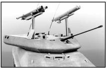
Below, the turret detail shows the pair of missile launchers in the raised position. One launcher is for antiaircraft missiles, the other for antitank missiles, both Russian weapons.
