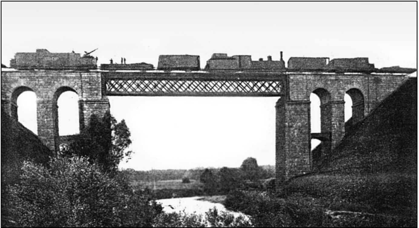
Although this train is Swedish, it is typical of those employed by many European armies and factions in the years before and after WWI. This view clearly shows the train's make-up, with the vulnerable engine in the middle, protected by a leading flatcar that will set off any mines. The cannon is visible in elevation on the armored car at left.
