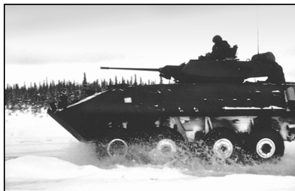
An LAV under test at the Cold Regions Test Center.
