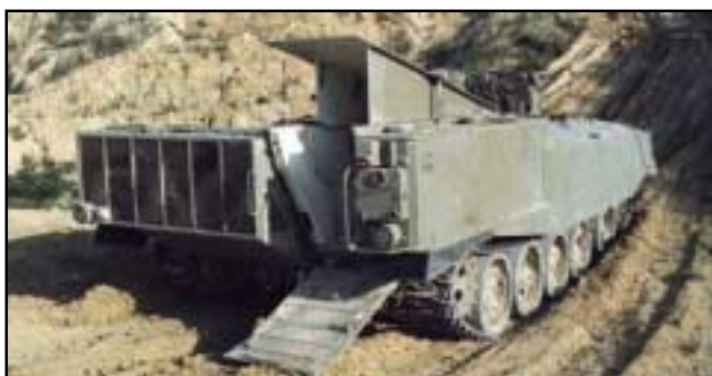
Israeli Achzarit heavy APC, at left and above, is based on a T-55 tank hull with the engine repositioned to create space for a clamshell door exit at the rear, as seen in the open position in photo at right.
