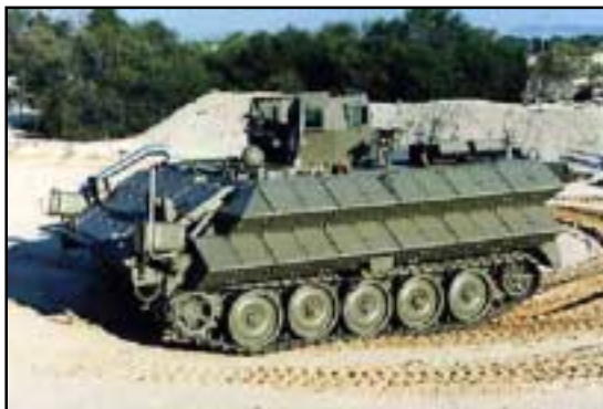
Up-armored Israeli M113, at left, has been equipped with explosive reactive armor (ERA) to enhance its protection against the shaped charge warheads of missiles and RPGs.
