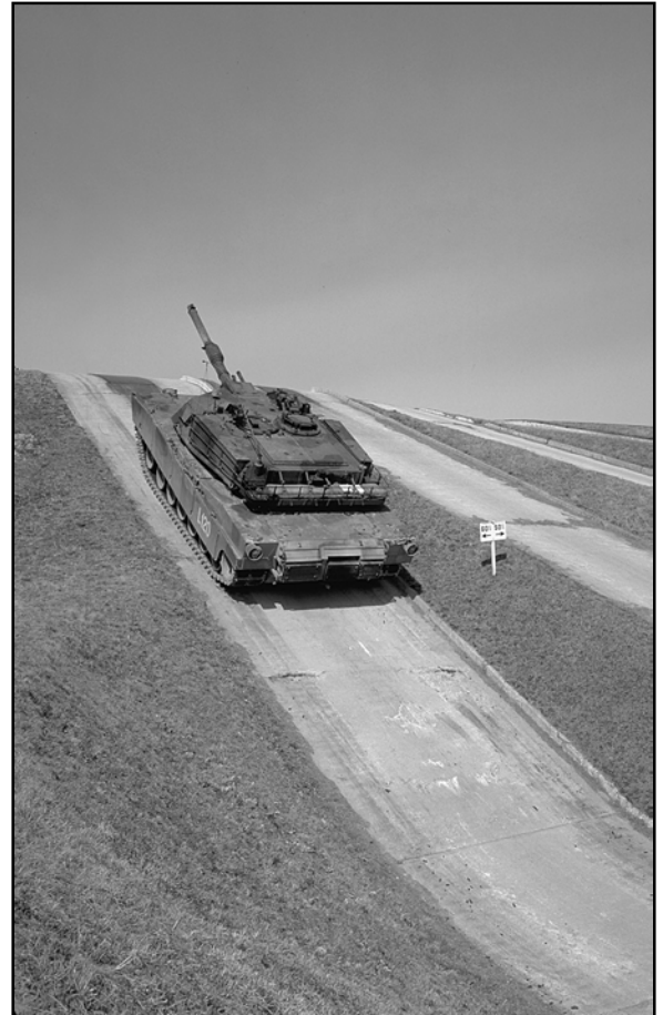
An M1A1 tank undergoes automotive testing on a vertical slope grade at the Aberdeen Test Center.
