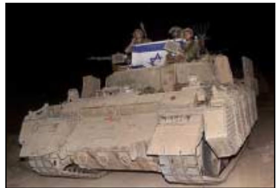
Up-armored Israeli M113, at left, has been equipped with explosive reactive armor (ERA) to enhance its protection against the shaped charge warheads of missiles and RPGs.
