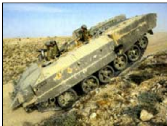
Israeli Achzarit heavy APC, at left and above, is based on a T-55 tank hull with the engine repositioned to create space for a clamshell door exit at the rear, as seen in the open position in photo at right.
