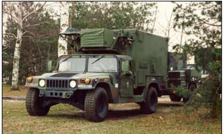
Mounted on a HMMWV, the Common Ground Station processes data from multiple sensors, including the J-STARS E-8C aircraft, unmanned aerial vehicles, and other intelligence platforms. —Motorola Photo
