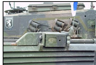
The Krauss-Maffei Wegmann rear-looking TV system allows the tank driver to move in reverse without assistance. The tiny camera, mounted in an armored box on the edge of the rear deck (see top photo), transmits a black-and-white image to a monitor in the driver's compartment.
