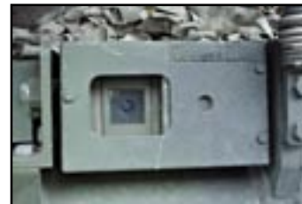
The Krauss-Maffei Wegmann rear-looking TV system allows the tank driver to move in reverse without assistance. The tiny camera, mounted in an armored box on the edge of the rear deck (see top photo), transmits a black-and-white image to a monitor in the driver's compartment.
