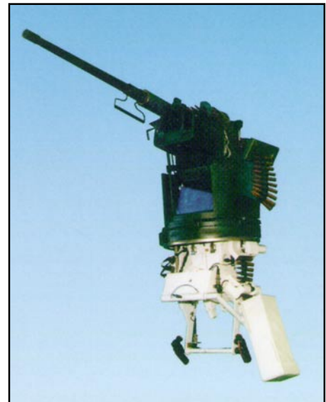
Israel’s Rafa’el is one of several firms manufacturing overhead weapons systems that can be fired accurately from within a vehicle. At left is their 7.62 MG system, and at right is the .50 caliber version.
