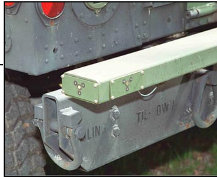
AAI Corporation’s Projectile Detection and Cueing system tells the crew where incoming fire is coming from. The sensors, seen above left on the bumper of a HMMWV, feed information to the monitoring screen, at right. In this case, fire is coming from the right front.
