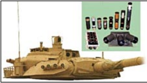
The French Galix grenade launching system. — Giat Photo
