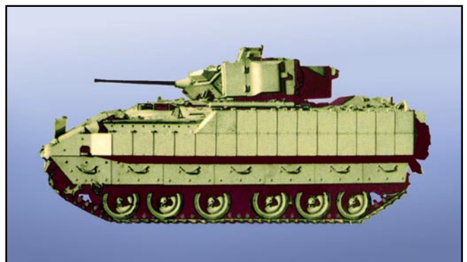
Rafa'el and Lockheed-Martin have developed a Super Blazer reactive armor package for the Bradley Fighting Vehicle.
