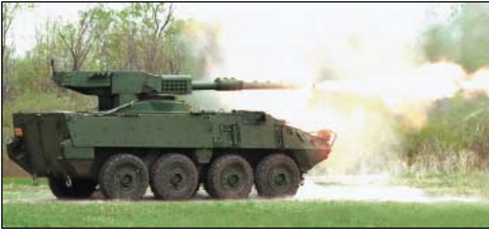
The Mobile Gun System firing its 105mm cannon in a firepower test. The cannon is a low recoil version of the L68 cannon that equipped the M60 and early M1-series tanks.
