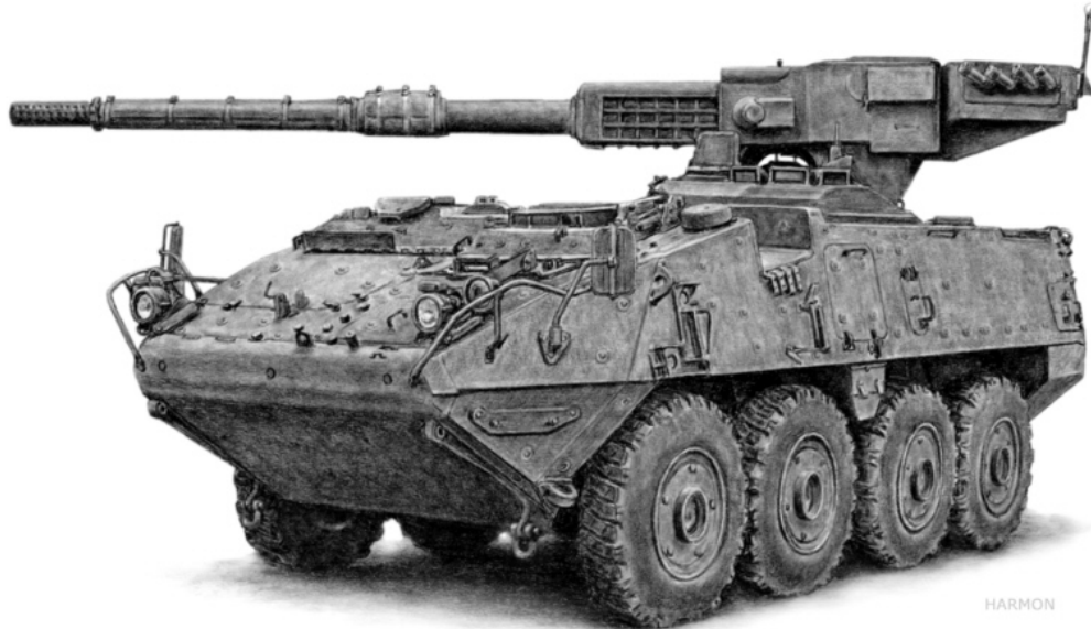
The LAV-based Mobile Gun System mounts a low-recoil 105mm cannon on the LAV's eight-wheeled chassis.
