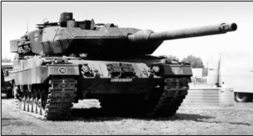
Above, a prototype of the Leopard 2A6, with its longer gun tube, seen here at the 1998 Eurosatory arms show.
