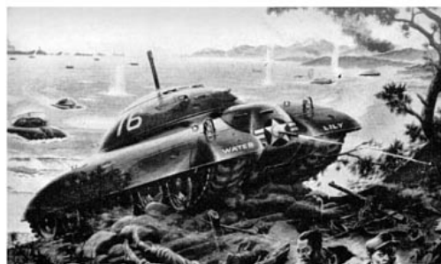
Arms are 105mm recoilless, flame thrower and machine guns, turret mounted.
