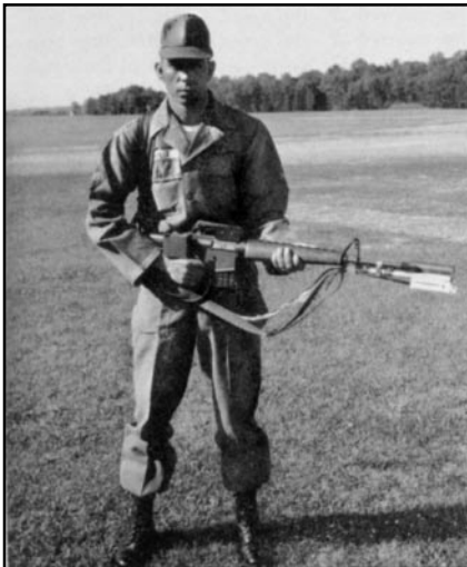
Front view of the Man Pack Prototype Chemical Personnel Detector with M16 Rifle.
