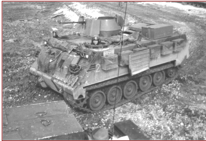
An ACAV kit on an M113, with improvised spaced armor made from empty ammo cans.
