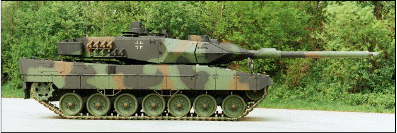
The Leopard 2A6 has a longer gun tube and new ammo.
