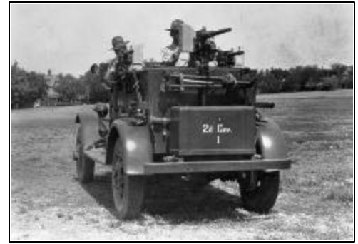
Prior to WWII, the Army purchased armored scout cars, like the one above, to perform reconnaissance, but the lowly jeep became the most common scout vehicle during the conflict. Another improvised solution, below, was an M5 light tank with its turret removed and replaced with a .50 cal. machine gun on a ring and trolley mount.
