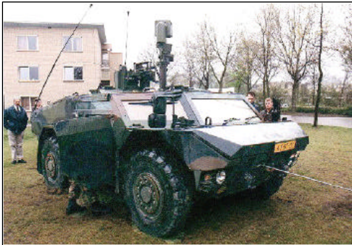
The “Fennek” (Desert Fox) reconnaissance vehicle carries a three-member scouting team equipped with mast-mounted FLIR, TV camera and laser rangefinder, powerful radios, and storage for enough supplies to sustain a 5-day mission.
