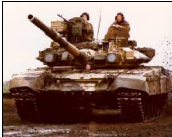
The Russian T-90, newly standardized by the Russian Army, features explosive reactive armor protection and a self-defense suite to protect against infrared-guided weapons. This model is based on the T-72 series.
