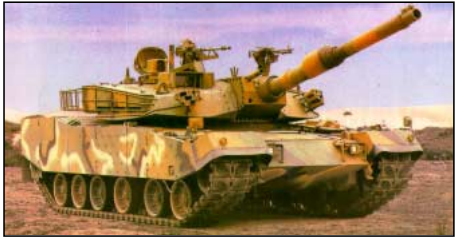
The Korean Type 88/120 "Baby M1" has been upgunned to 120mm from 105mm.
