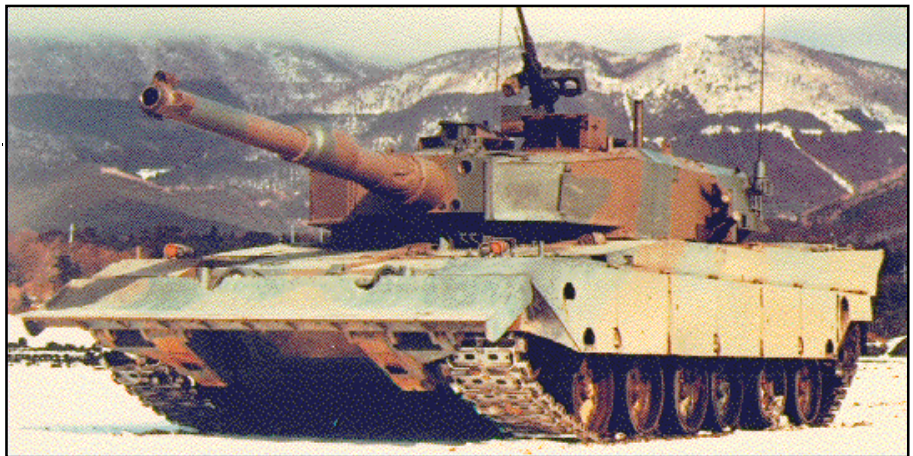
The Japanese Type 90 is armed with the same German-developed gun as the U.S. Abrams. Its vehicle electronics reflect the advanced technology of Japanese industry.
