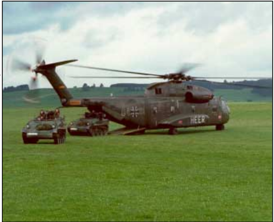
The German Army uses Wiesel armored weapon carriers, which are helicopter-deployable, as the core of a light armored battalion. They can be armed with 20mm autocannons or TOW missile launchers. The limited internal space, however, rules them out as carriers of a four-man scout team with its equipment, and Wiesels are not amphibious. – MAK Photo
