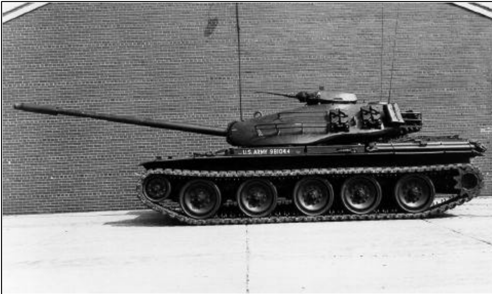
Pockets in the turret casting of the U.S. T-95, an experimental tank, were filled with fused silica, a form of quartz sand, as an element in the tank's armor protection. It was believed that the silica would protect against HEAT warhead penetration and be no worse than steel armor in defeating kinetic energy attacks. Note also that the track system had no return rollers.
