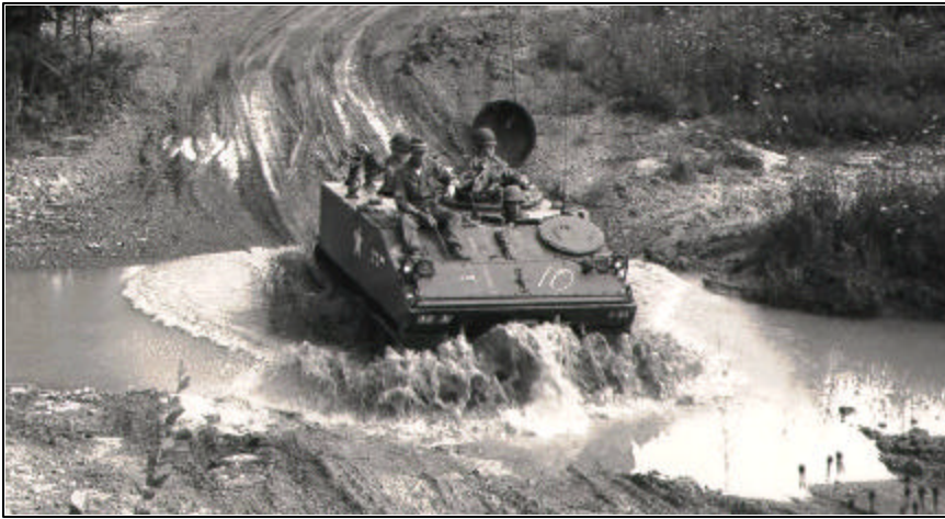
The M114 APC above, was another misdirected attempt at a scouting and reconnaissance vehicle. Seen here crossing a ford in tests at Fort Knox, it was less successful crossing paddy dikes in Vietnam, and was withdrawn from service.
