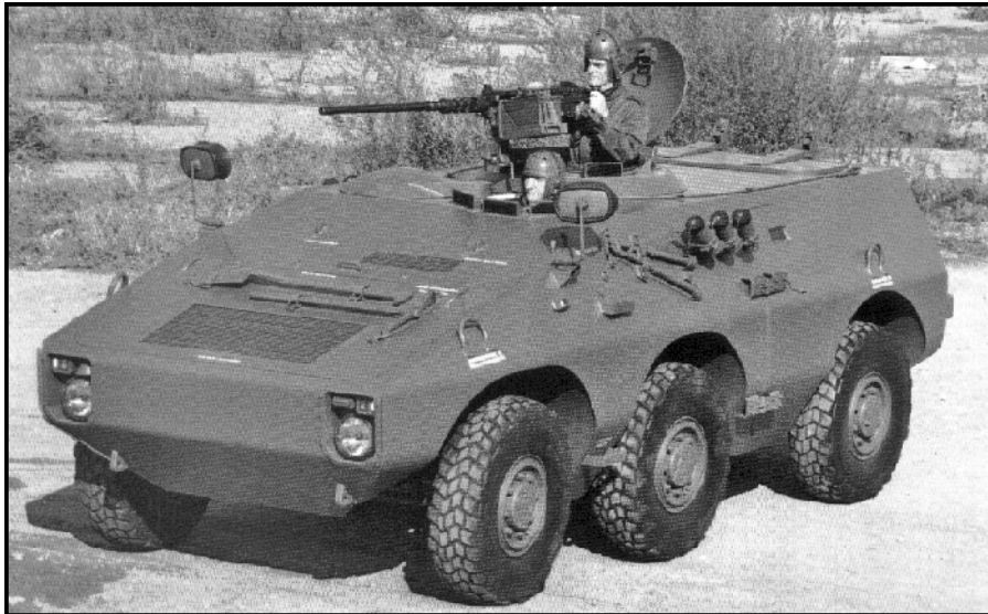
This is the 6x6 version of the Puma, under consideration as a troop carrier to accompany the Centauro armored car in cavalry units.
