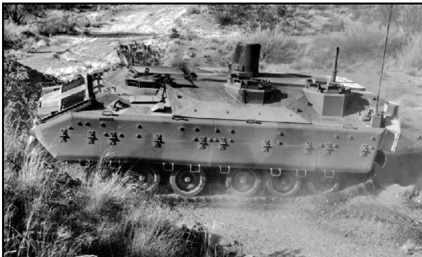
The shape of things to come? A missile-armed Future Combat System might resemble the Bradley-LOSAT prototype shown here. A very low silhouette is made possible by a turretless configuration. (Photo: Loral Vought Systems)
