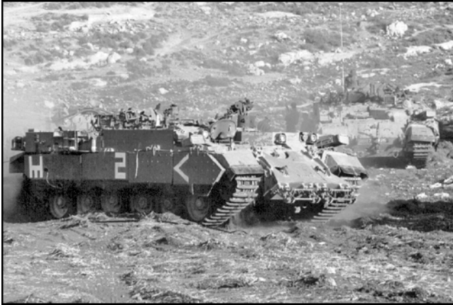
Above, an IDF "Puma," a Centurion tank modified as an armored personnel carrier. At right, the Magach-8, an M60 variant with a modular armor suite offering protection similar to the Merkava.
