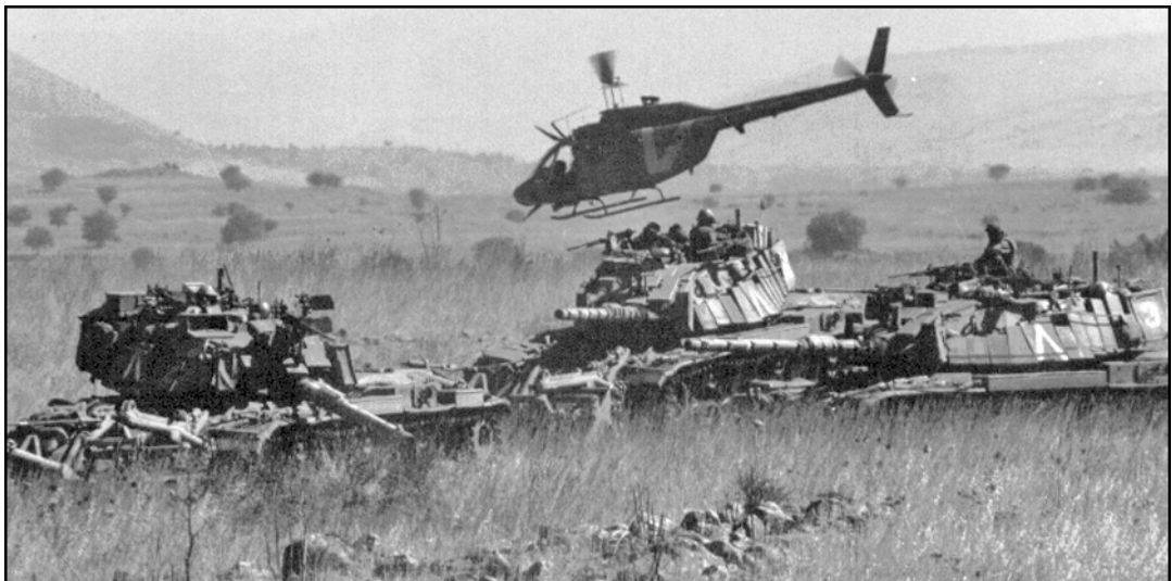
Above, an IDF "Puma," a Centurion tank modified as an armored personnel carrier. At right, the Magach-8, an M60 variant with a modular armor suite offering protection similar to the Merkava.
