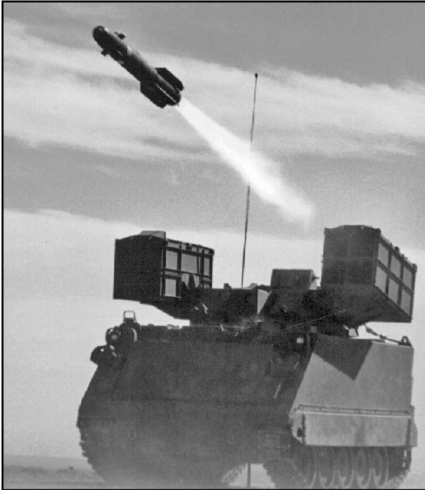
Hellfire, seen here being fired from an M113, can hit targets as far away as 8000 meters—almost three times as far as the Abrams! If adapted to the Longbow Hellfire system, ground forces would have a heretofore unknown combat capability. (Photo: Rockwell International)
