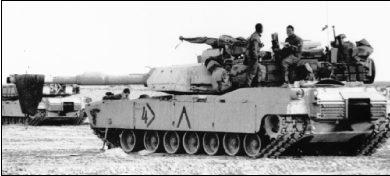
An M1A1 crew from 1-35 Armor pauses during Desert Storm. Note the external turret stowage space unavailable in an EGT design.
