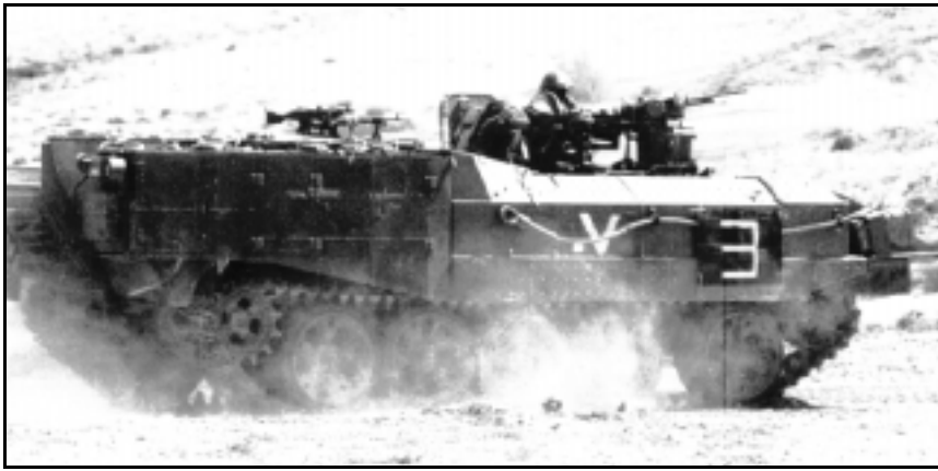
A heavy armored personnel carrier, based on a captured T-55 chassis. The turret has been removed, the engine compartment has been redesigned, and a hatch has been added to the rear for troop access. Other obsolete tanks have been converted to engineer vehicles.
