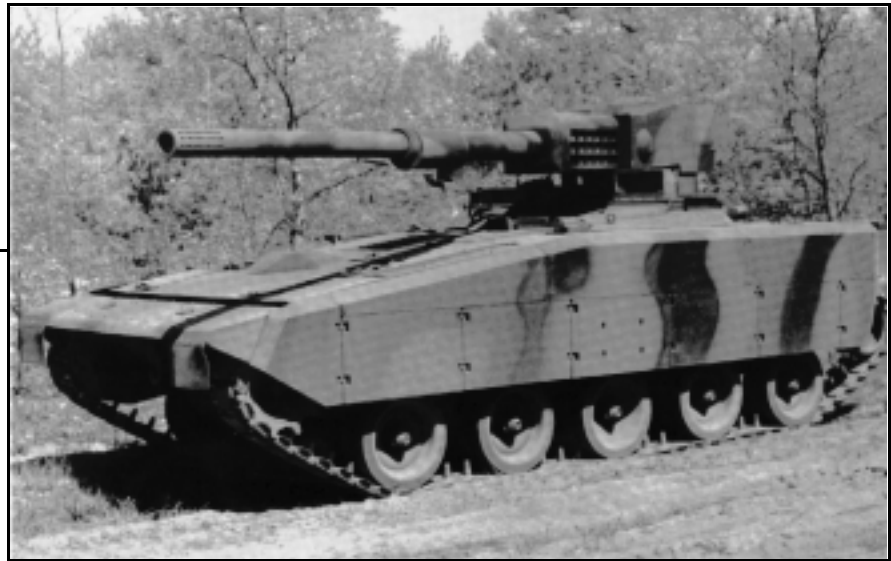
Among many vehicles that have explored the concept of external guns were the General Dynamics Armored Gun System candidate, above, and the HIMAG (High Mobility Agility) vehicle, shown at left being tested in 1980.
