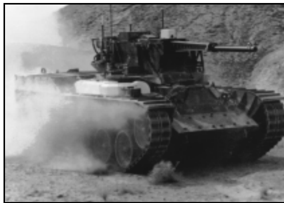
Among many vehicles that have explored the concept of external guns were the General Dynamics Armored Gun System candidate, above, and the HIMAG (High Mobility Agility) vehicle, shown at left being tested in 1980.
