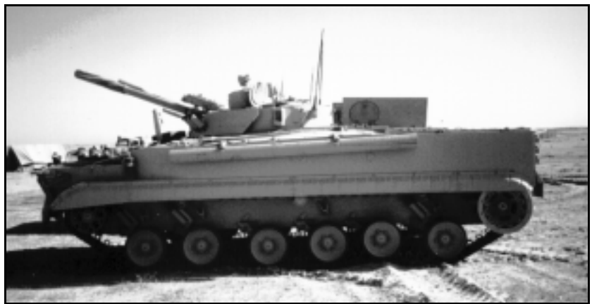
Left side view of the BMP-3. Note laser rangefinder over main gun mantlet.
