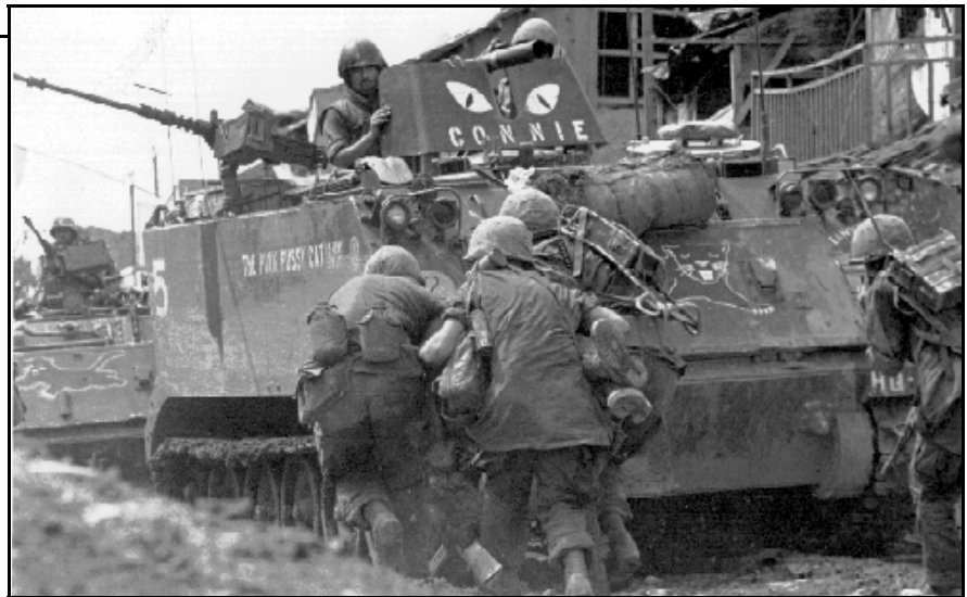
Soldiers carry a wounded man to the safety of an M113 ACAV during fighting in Saigon in 1968. The vehicle's armament includes a pintle-mounted .50-caliber machine gun firing over the right side and a recoilless rifle in the front ACAV turret.
