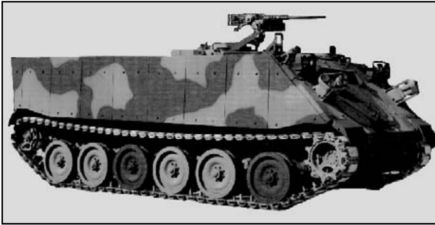
The Mobile Tactical Vehicle Light (MTVL), latest derivative of the M113 family, as seen in a United Defense brochure. The most recent improvements include a 350-hp turbocharged engine and an improved suspension that allows more than 15 inches of roadwheel travel. The M113 is probably the most common armored vehicle in the world.
