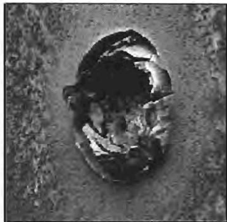
Figure 2. Exit hole created by the same explosively formed penetrator. When this photograph was taken, the metal surrounding the hole was still crackling and sizzling from the heat produced by the penetrator.
