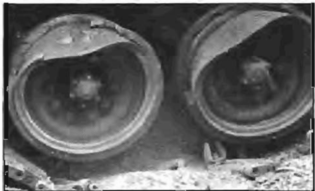
Figure 4. Damaged road wheels and track caused by a track-width AT mine. This type of mine is activated by the ground pressure exerted by an armored vehicle.
