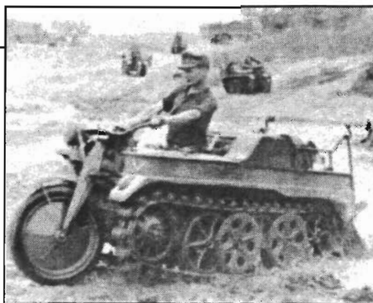
Similar to a halftrack, the German Kettenrad motorcycle had a track-laying system instead of a rear wheel.
