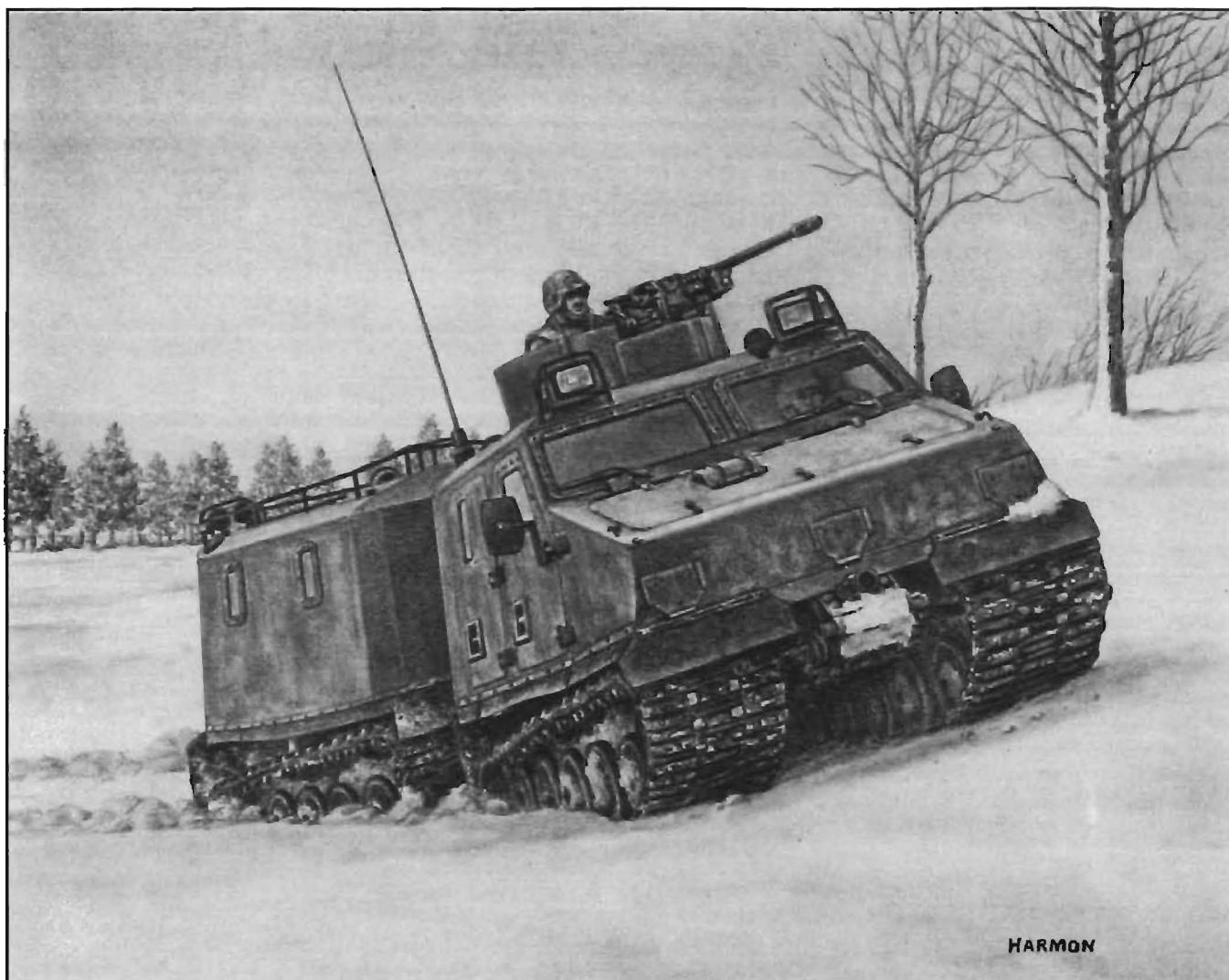
Figure 1. Artist's conception of a Hagglunds Armored All-Terrain Carrier configured for scout use.
