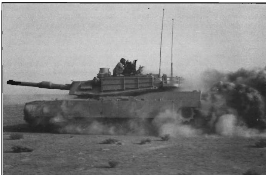
Above and at right, the Abrams tackles the soft sand slope test in its mobility demonstration. The competing British Challenger II had difficulty in this test. Below, the Abrams demonstrates its speed racing across the desert in another evaluation of the tank's mobility. Kuwait, Saudi Arabia, and the United Arab Emirates are all in the market for new main battle tanks and are evaluating the British DESERT STORM veteran and the improved version of the U.S. tank. The UAE recently indicated it may choose a third contender, the new French Leclerc MBT.
