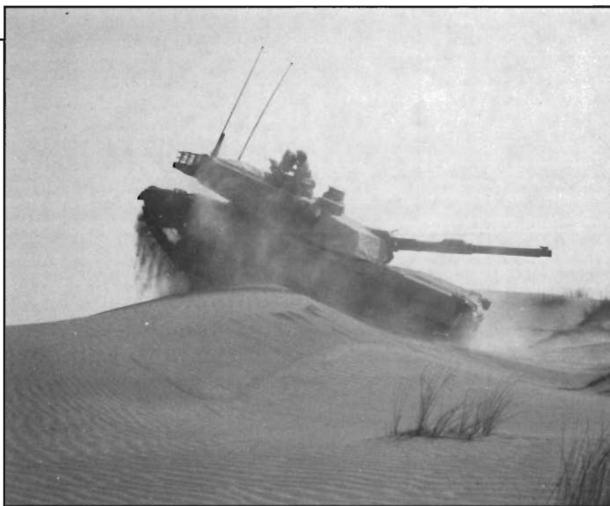
Above and at right, the Abrams tackles the soft sand slope test in its mobility demonstration. The competing British Challenger II had difficulty in this test. Below, the Abrams demonstrates its speed racing across the desert in another evaluation of the tank's mobility. Kuwait, Saudi Arabia, and the United Arab Emirates are all in the market for new main battle tanks and are evaluating the British DESERT STORM veteran and the improved version of the U.S. tank. The UAE recently indicated it may choose a third contender, the new French Leclerc MBT.
