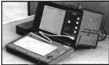
CTS III diagnostic computer, above, which is linked to the tank engine by a 129-pin connector through an RS-232 port. Connectors and circuit boards are at right.
