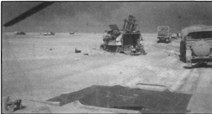
This AAVP7A1 with Mark 154 mine-clearing system, similar to the MICLIC, itself hit a mine in the breaching of the Iraqi defenses.
