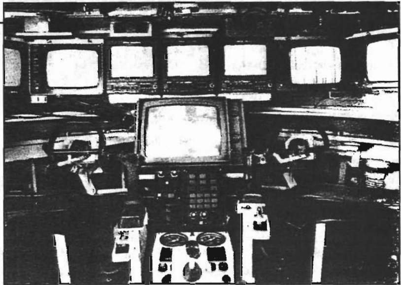
Array of TV screens needed for 360-degree viewing in German VT 2x2 test vehicle.
