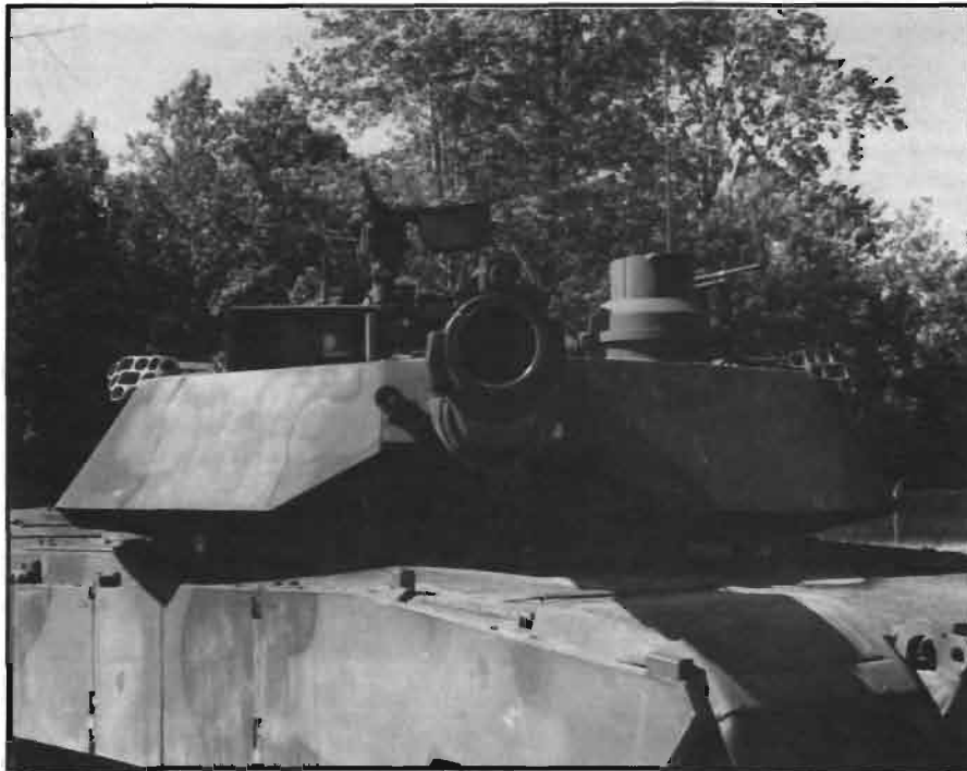
CITV dome on left turret front identifies the M1A2 version.
