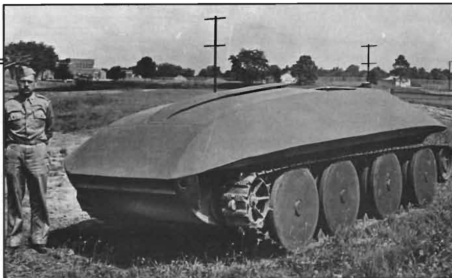
The rejected Bigley vehicle, as tested in 1942, and considered by the Palmer Board, with mock-up body. (Icks Collection: Patton Museum)
