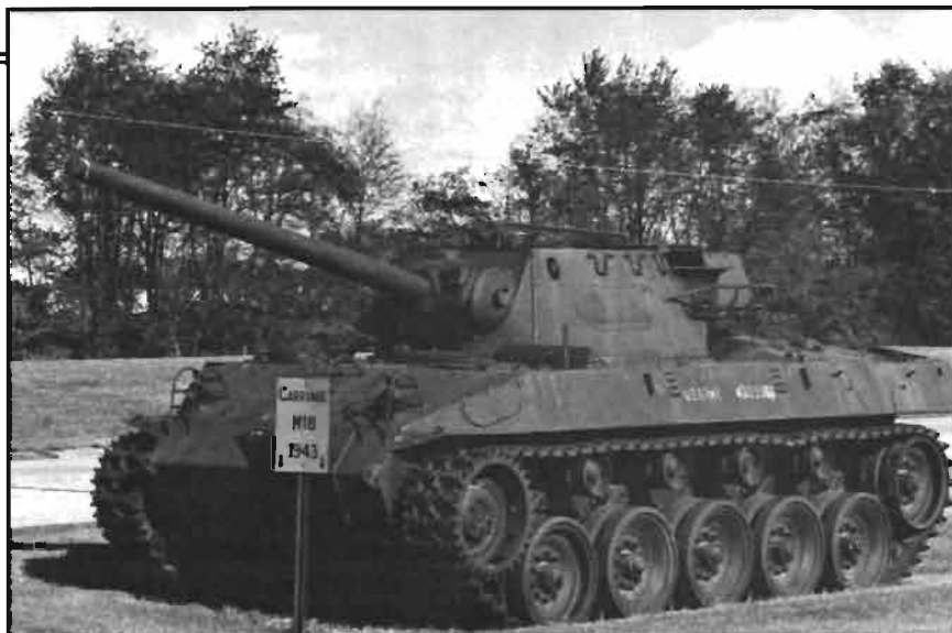
After examining and rejecting Christie's coil-spring suspension, Ordnance decided to use the torsion bar system on the M18 "Hellcat" tank destroyer.
