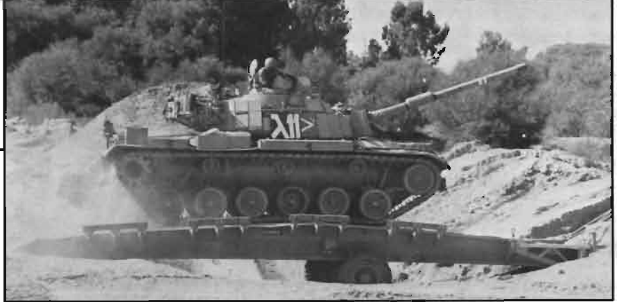
Wheeled assault bridge is pushed across a trench by an M60 tank. This bridge can be attached to any tank, so the unit does not depend on heavy, dedicated bridgelayer tanks. The tank attached assault bridges are inexpensive and can be left on location for long periods, if required
