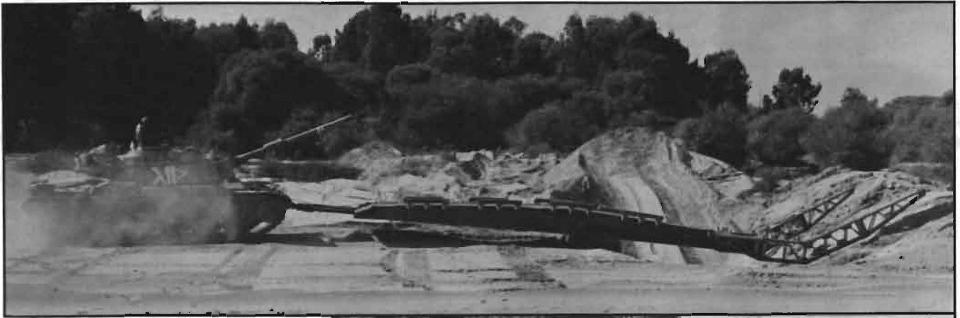
Wheeled assault bridge is pushed across a trench by an M60 tank. This bridge can be attached to any tank, so the unit does not depend on heavy, dedicated bridgelayer tanks. The tank attached assault bridges are inexpensive and can be left on location for long periods, if required
