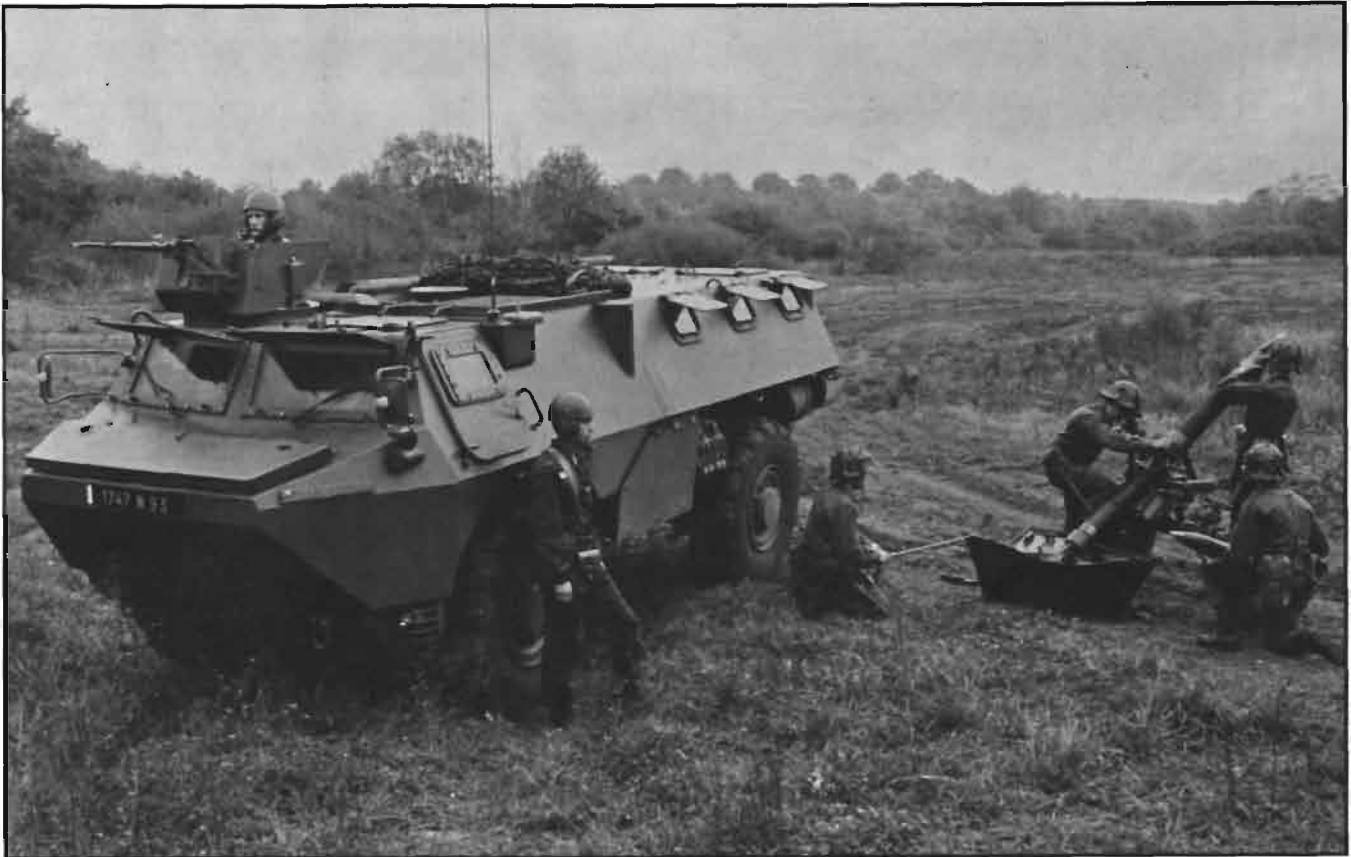
This French Army VAB 4x4 is a 120-mm towed mortar crew vehicle.
