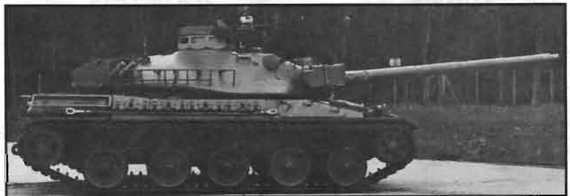
AMX-30B's low-light TV camera is on the right side of the turret.
