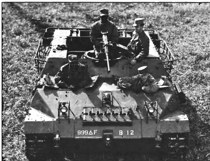
The forerunner of later armored personnel carriers, the M39 - seen here in a postwar exercise - was based on the M18 Hellcat chassis. It saw little action in WWII.
