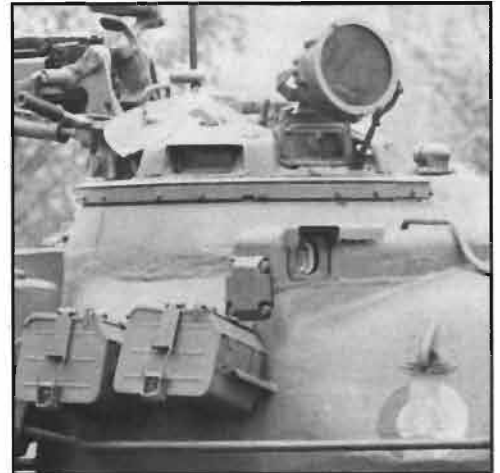
T-72B has right side window for earlier coincidence rangefinder. This one is East German.
