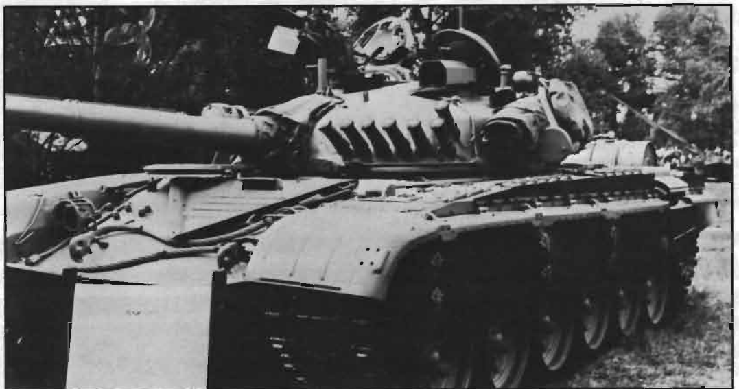
T-72M1 resembles the G Model, but has an add-on armor plate covering the front slope. Tow hooks pass through add-on plate. This T-72M1 is Finnish.
