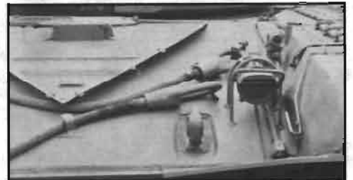
Close-up shows add-on armor plate on T-72M1 front slope and tow hook openings.
