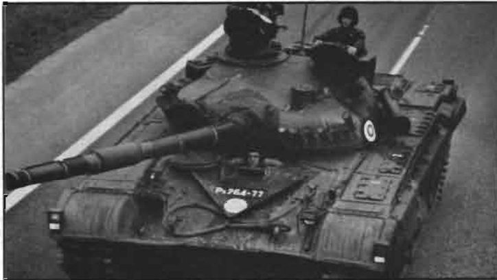
T-72M1 resembles the G Model, but has an add-on armor plate covering the front slope. Tow hooks pass through add-on plate. This T-72M1 is Finnish.
