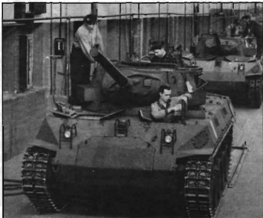
M18 Hellcat tank destroyers being assembled at the GM Buick plant in Flint, Michigan. Like the M26 and M24, the M18 had torsion bar suspension. The M18 could do 75 MPH.
