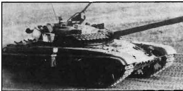
T-64B with reactive armor attachment points
