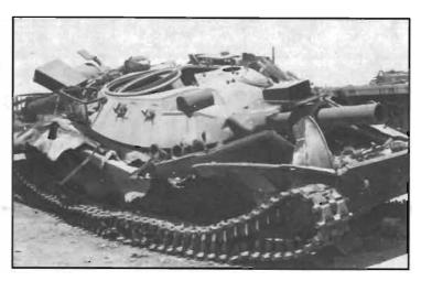
This M151 Sheridan AR/AAV, seen in a salvage yard in Vietnam, was destroyed by an antitank mine and the secondary explosion of its own ammunition. Current research is directed at preventing secondary fuel and ammunition fires.
