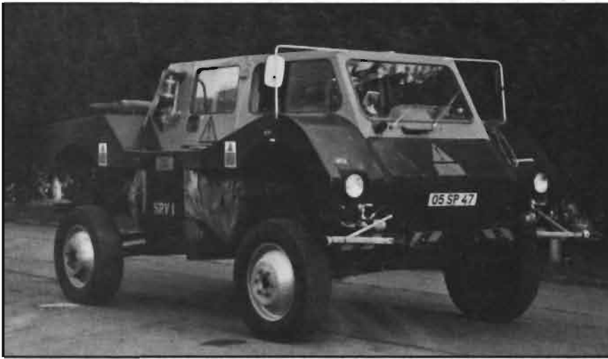
Special research vehicle with large wheel movement used to study active suspensions.
