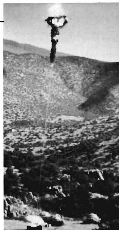
"Smart" indirect-fire weapons, like the SADARM, seen in tests, above, attack weak top armor.
