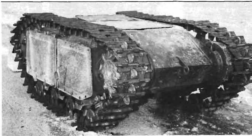
The "Goliath", a German WWII invention, was controlled by a trailing cable, carried up to 125 pounds of high explosives, and was intended to destroy fortifications and clear minefields. It was not very successful.
