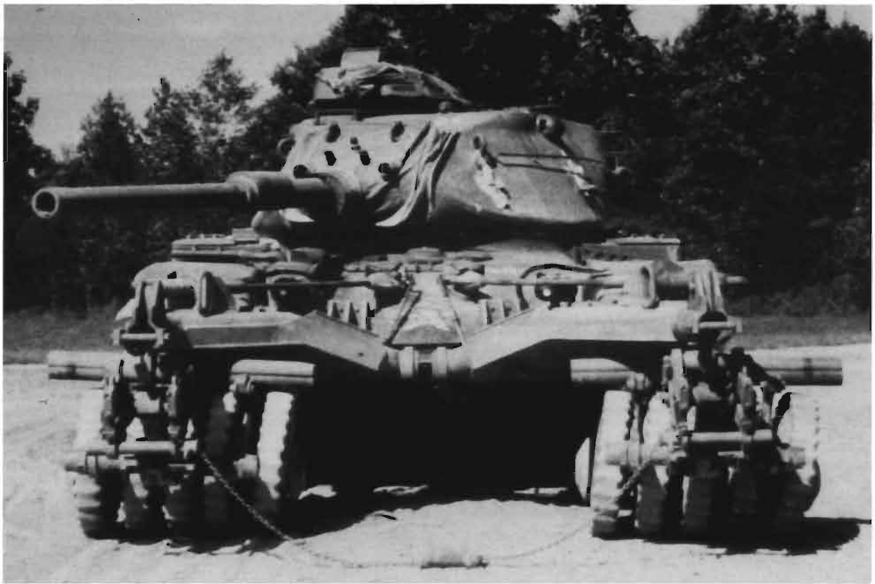
Current Tracked-Width, Tank-Mounted Mine-Clearing Roller evolved after a long period of experimentation beginning in WWII.
