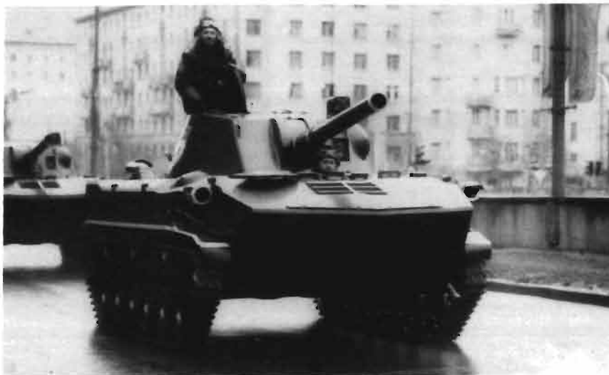
Two views of the mortar-howitzer variant of the BMD reveal points of difference: the longer hull, extra roadwheel, and new turret. View of top of the hull, at right, shows driver's central position in the hull. The author notes the asymmetric blister on left front of the turret, possibly part of the vehicle's fire control.
