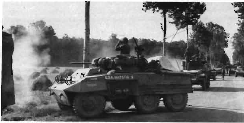
The U.S. made widespread use of wheeled armor during WWII, which paid off during high-speed exploitations in Europe. The M8, at left, mounted a 37-mm gun. The heavier (26 tons) Boarhound heavy armored car, seen below, was designed for desert fighting, but too late. It was never produced in large quantities or used by U.S. troops.
