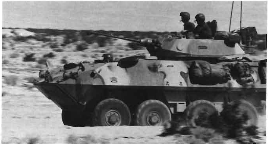
Above, the Marines maneuver with their new LAV, an 8-wheel armored vehicle with 25-mm cannon.
