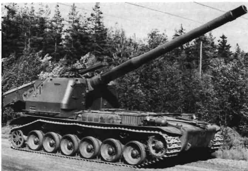
The Swedish Bandkanon IA self-propelled artillery piece has movable rear idlers which drop to stabilize the vehicle in firing position. Engine is in the front.
