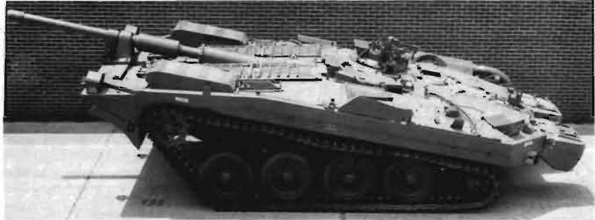
More "gun-in-hull" than "gun-over-hull," the Swedish S-Tank design was revolutionary in its time.
