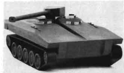
Model illustrates the Swedish UDES configuration with gun in raised position.
