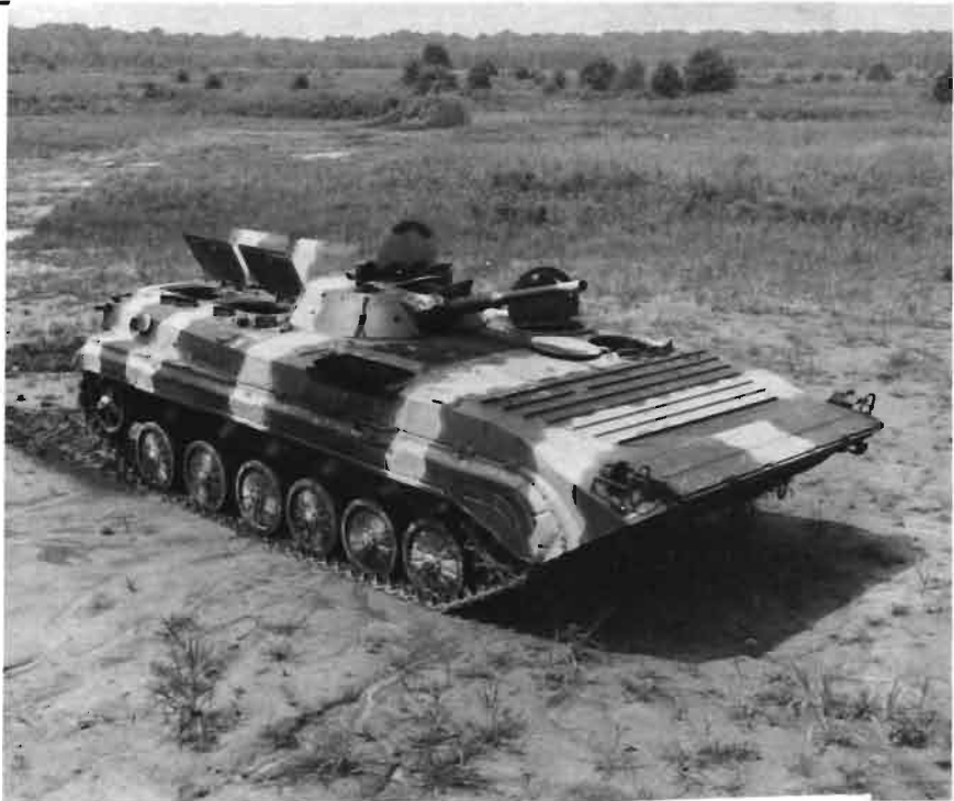
Comparison of this photo of the BMP-1 with the drawing of the BMP-2, opposite page, indicates changes in rear deck hatches and reflects reduction in infantrymen carried inside the new model.
