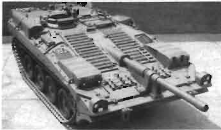
The Swedish "S" Tank, a 1960s design, exemplifies one type of casemate configuration, with the main gun fixed within the hull.
