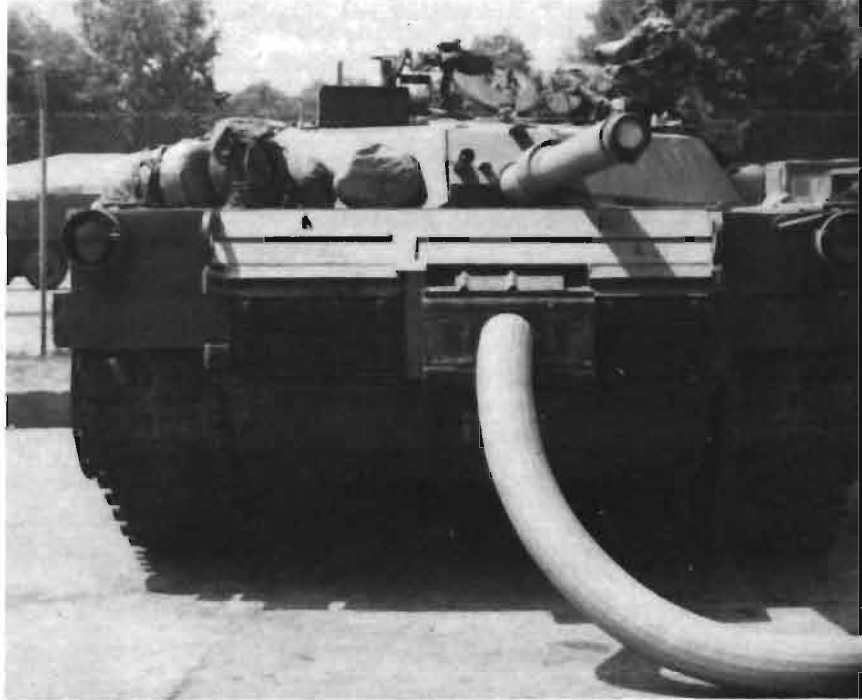
FIGURE 2. "Cannon Device" uses M1 turbine exhaust for decontamination.
