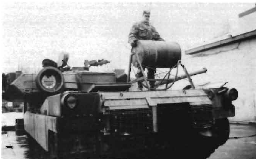
FIGURE 4. 55-gallon drum mounted on tank deck feeds decon solution to smoke generator.
