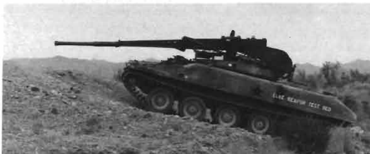
Shown being tested here on a Sheridan chassis, the Elevated Kinetic Energy Weapon (ELKE) features gun trunnions that go up on pivoting arms mounted at the turret rear.
