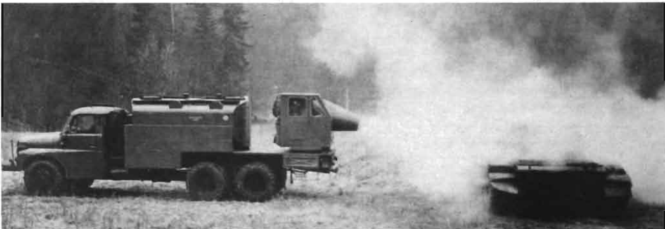
FIGURE 1. Russians have long used truck-mounted jet engines to decontaminate tanks, car-wash style.
