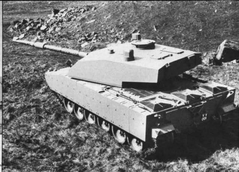
The Chobham-armored Vickers Valiant weighs in at 43.6 metric tons, some 10 tons, or more, lighter than the M1 . The four views show the main gun, armor array, and suspension system.
