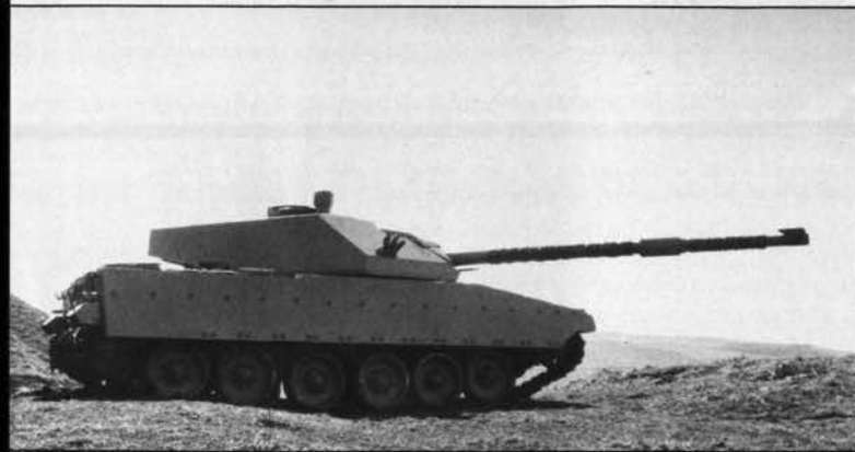
The Chobham-armored Vickers Valiant weighs in at 43.6 metric tons, some 10 tons, or more, lighter than the M1 . The four views show the main gun, armor array, and suspension system.
