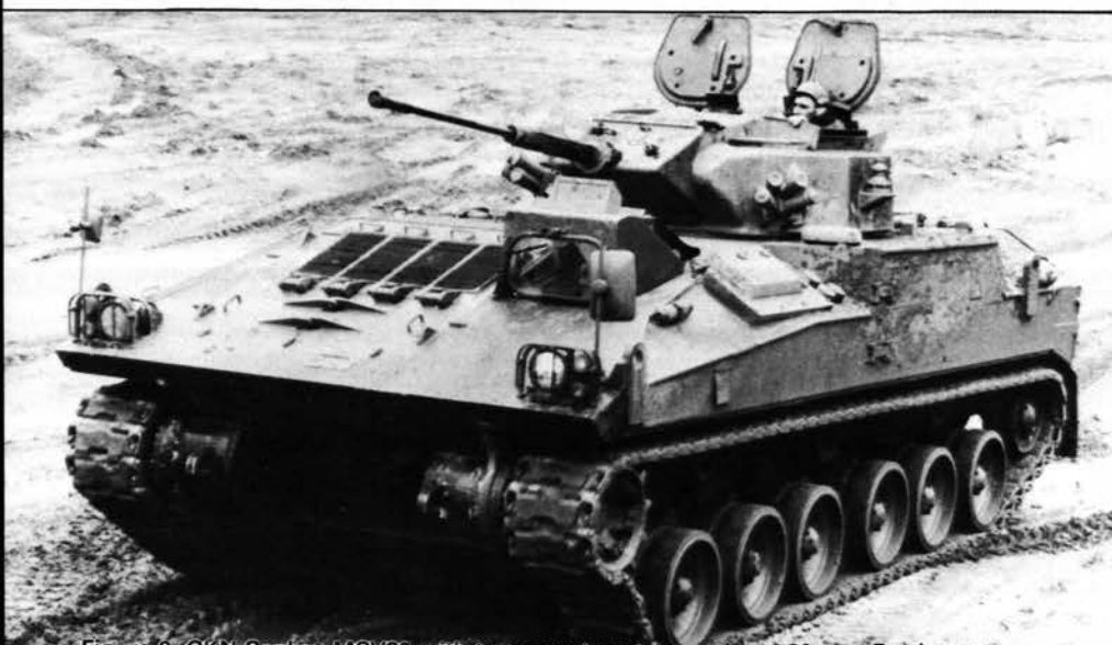
Figure 2. GKN-Sankey MCV80 with two-man turret mounting a 30-mm Rarden gun.
